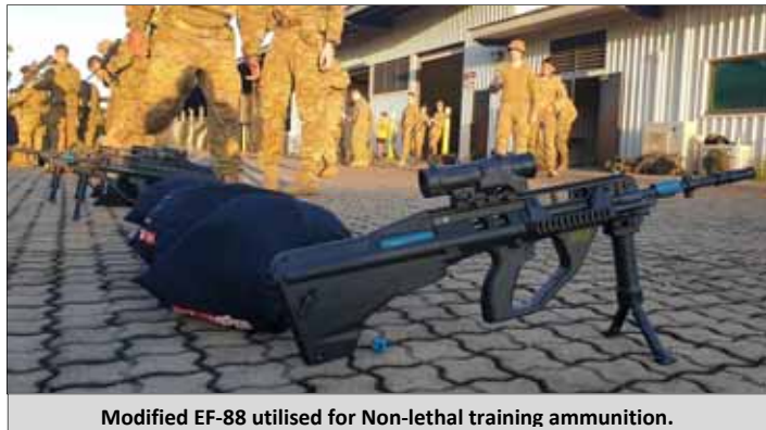
Modified EF-88 utilised for Non-lethal training ammunition.
