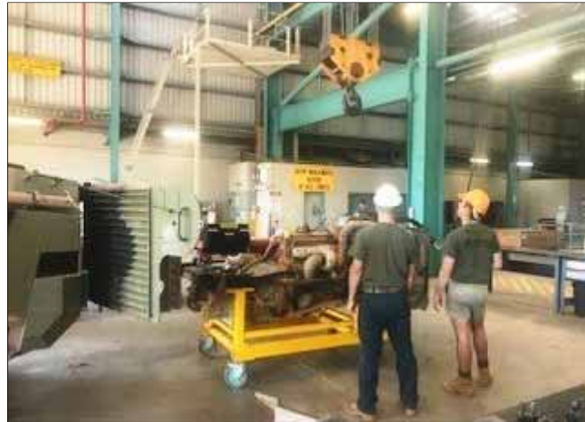
TSP Vehicle Section conduct the removal of a PMV power pack.
